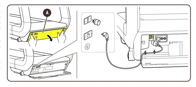
Fix the cable into the channel provided using the cable clamps supplied. Close panel (A) again, threading the cable through the slot provided.
