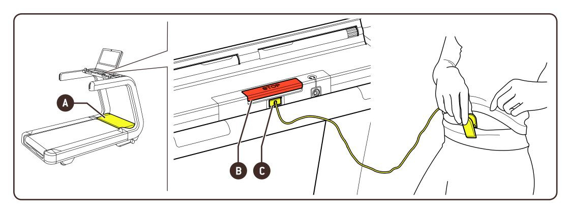
After finishing working out, put the emergency switch peg back into its slot, as shown in the illustration.
