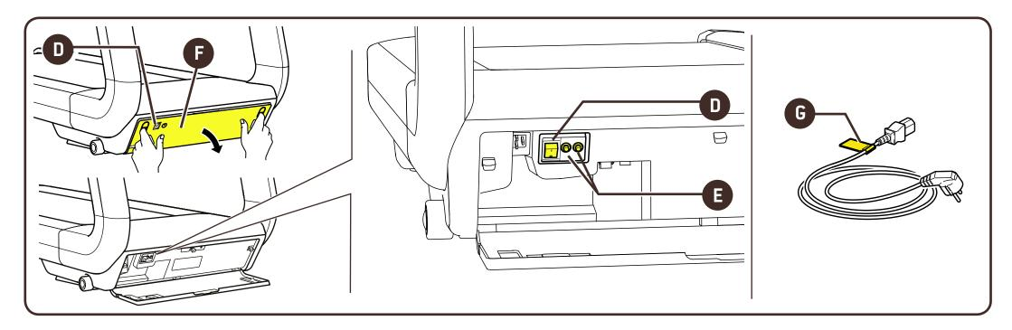
The label (G) which can be attached to the power supply cable states the electrical specifications for the cable.
